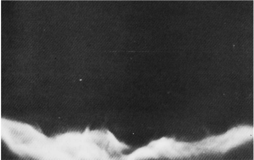
FIGURE 7. Variation of the density interface marked by fluoresceine dye by a vertical sheet of light parallel to the rotation axis. Experimental conditions are: \Omega = \pi \text{ rad s}^{-1} , S = 4 \text{ cm} , n = 6.6 \text{ Hz} . The distance of the interface from the grid midplane is D = 30 \text{ cm} . (a) \Delta\rho/\rho = 0.5\% , Ri = 4.5 ; (b) \Delta\rho/\rho = 1.5\% , Ri = 13.5 .
